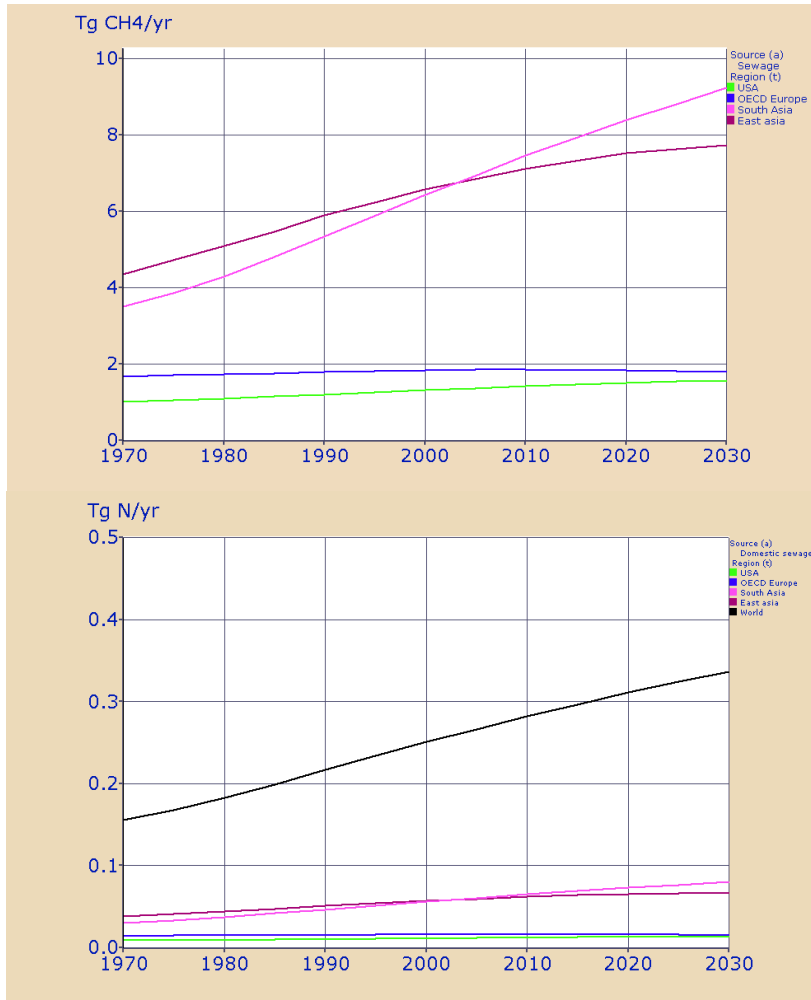
Figure 2.6b. Emissions of CH 4 (top panel) and N 2 O (bottom panel) from sewage for OECD Europe, USA, South Asia, East Asia and the world for the period 1970-2030 in the GECS baseline scenario.
