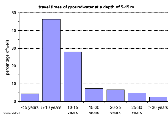
Figure 41: Travel times distribution of groundwater in the sand regions in the Netherlands at a depth of 5–15 m.
