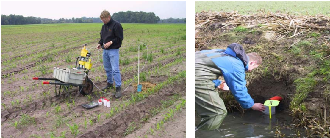
Fig. 13 Sampling of upper meter of groundwater in the sand regions (left) and of tile-drain water in the clay regions (right).
