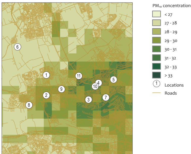
PM 10 GCN map for 2007. The monitoring locations from the Osiris campaign are represented by the dots and numbers.
