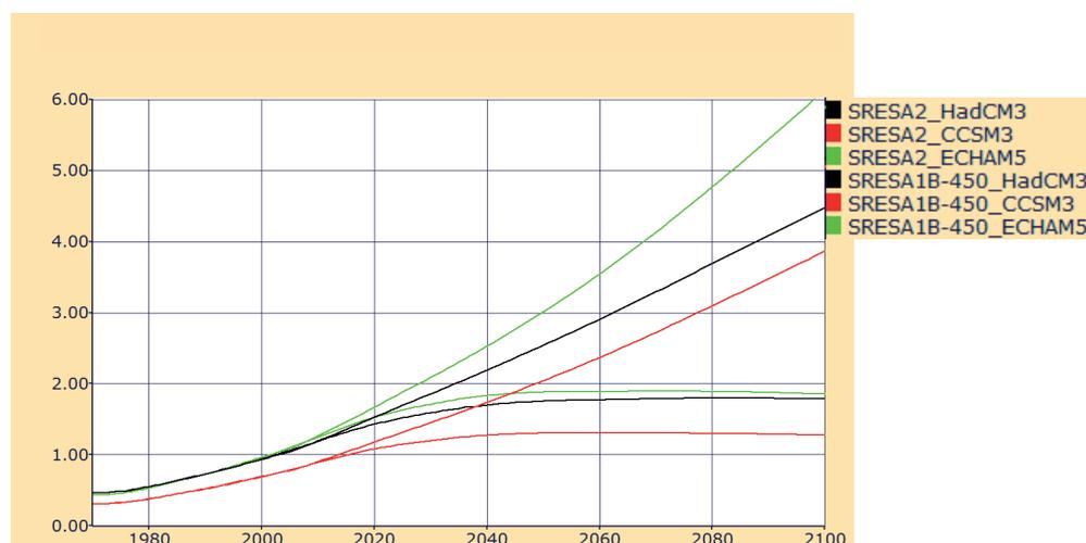
Mean global near-surface air temperature change in the SRES A2 (top lines) and SRES A1B-450 (lower lines) scenarios, in IMAGE 2.5, with various parameter settings emulating the behaviour of HadCM3 (black), CCSM3 (red) and ECHAM5 (green).
