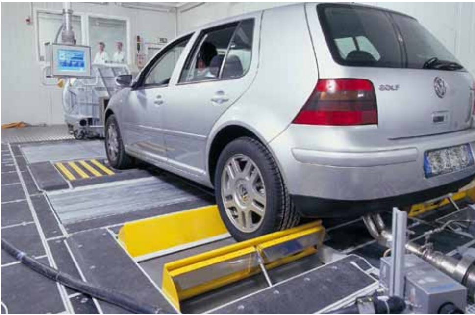
Photo 6 Emission testing of cars running on biofuels blends is important in monitoring effects on air polluting emissions. Test facility for light duty vehicles at Joint Research Centre in Ispra, Italy © EC (2009)
