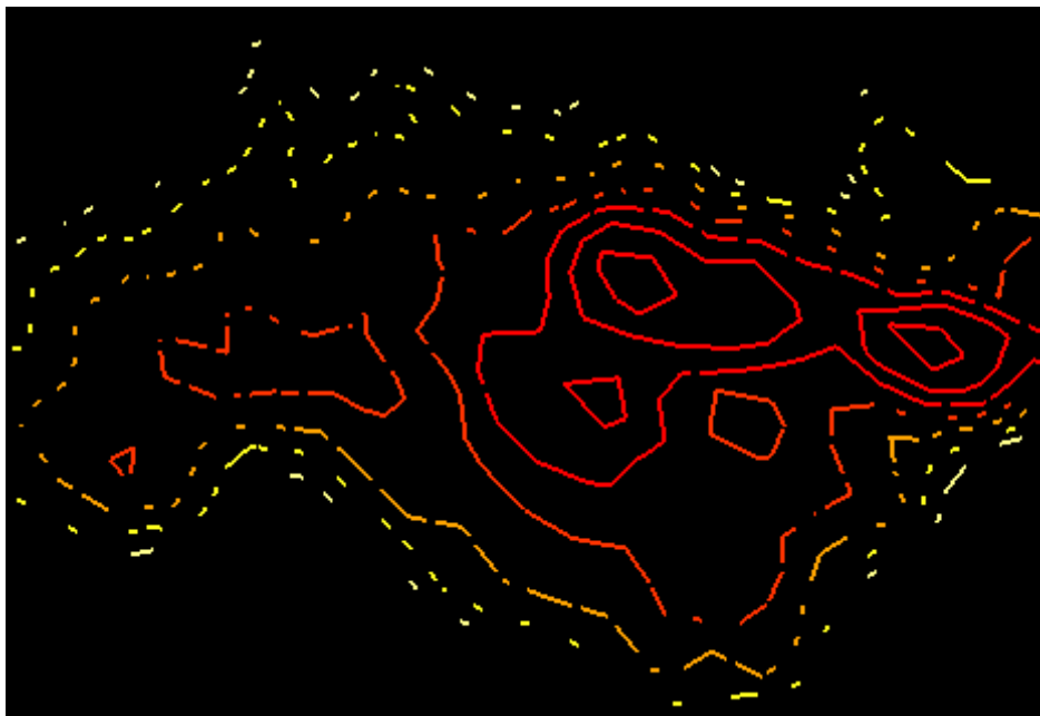
Figure 21 Spatial uncertainty is encoded as gaps in contour lines. The more uncertainty, the larger the gaps [22].
