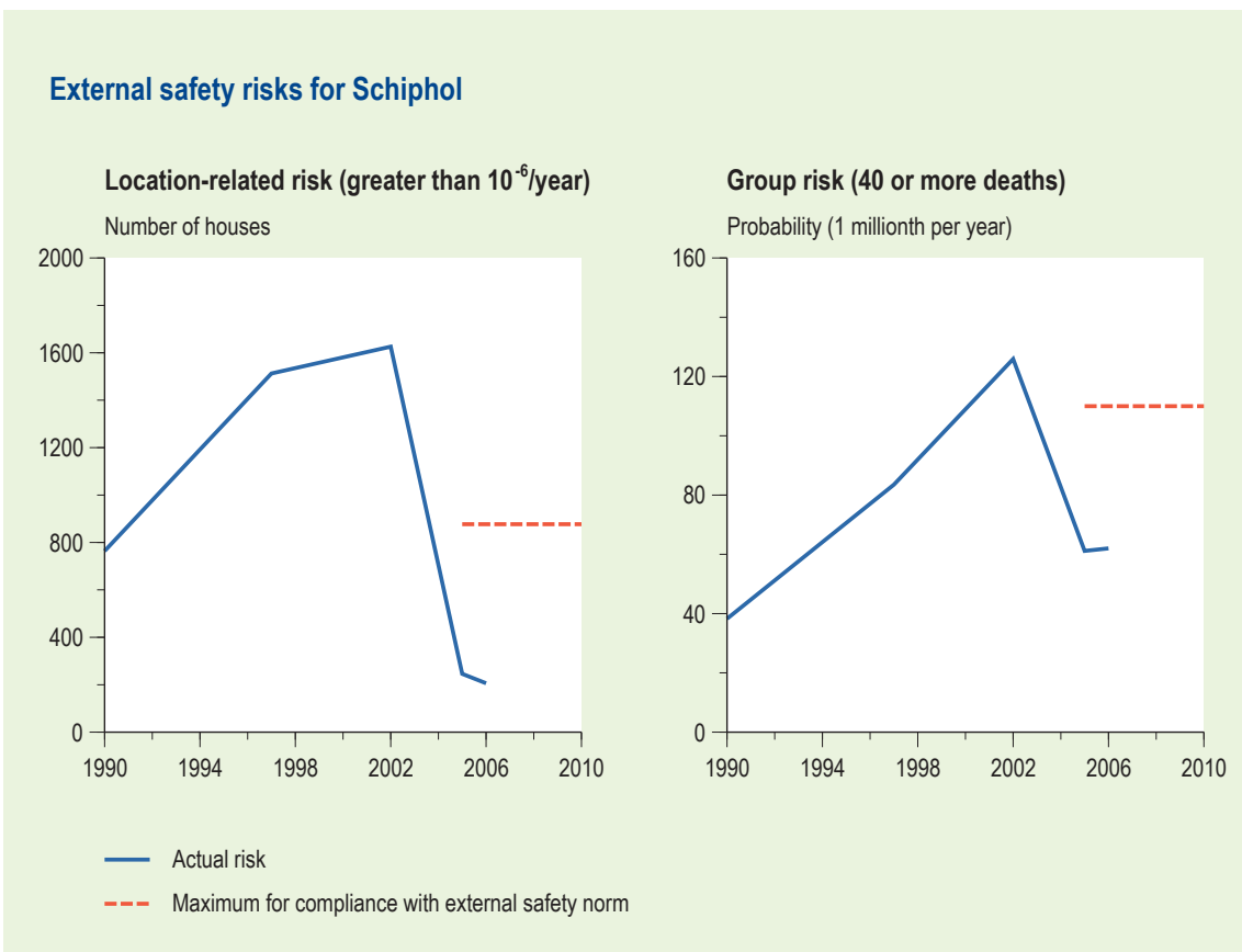
Figure 2.13 Development of location-related risk (left) and group risk (probability of a disaster with more than 40 victims) (right) from air traffic around Schiphol. Calculations for all years are based on actual volumes of air traffic.
