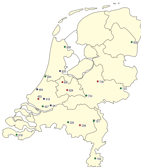
Figure 2.3 Monitoring sites for the determination of PM 10 (Van Elzakker, 2000). The blue points are urban background stations, the green points regional background stations and the red points street stations. The numbers and corresponding names of stations can be found in Table 2.3.
