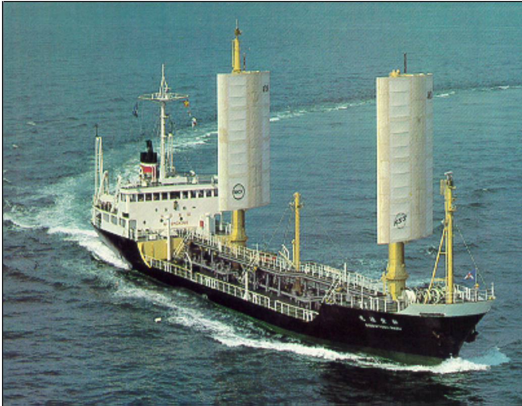
Figure 4.3.1: “A tradeable CO 2 permit system promotes technology developments such as illustrated by this Japanese ship. “The sail on the fully loaded ship can provide 53% of the power to travel 12 knots. To get the most from wind speed and points of sail, a microcomputer gives automatic commands to trim the steel-framed canvas sails by rotating the masts. With efficient equipment and design, fuel savings can be as high as 50%. The incentive: Japan’s acute need to conserve imported oil” [during the oil crises] (source: National Geographic, February 1981).
