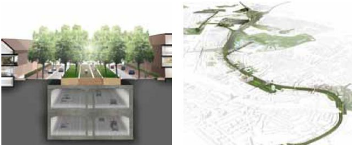
Figure 2. A tunnel has been designed under the part of the A2 motorway that runs through Maastricht, with a green belt along it, on surface level, to be used for recreation (figure on the left). This green belt operates as an ecological connection between a number of large nature areas (figure on the right). Private parties are also involved, partly because of the expected increase in value of the real estate in the vicinity of this green belt.
