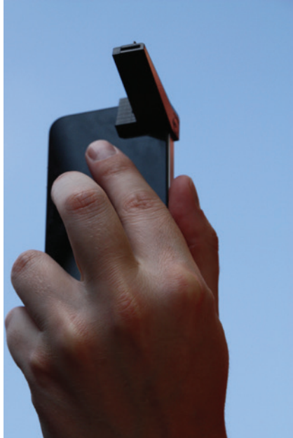
iPhone with device for measuring particulate matter concentrations
