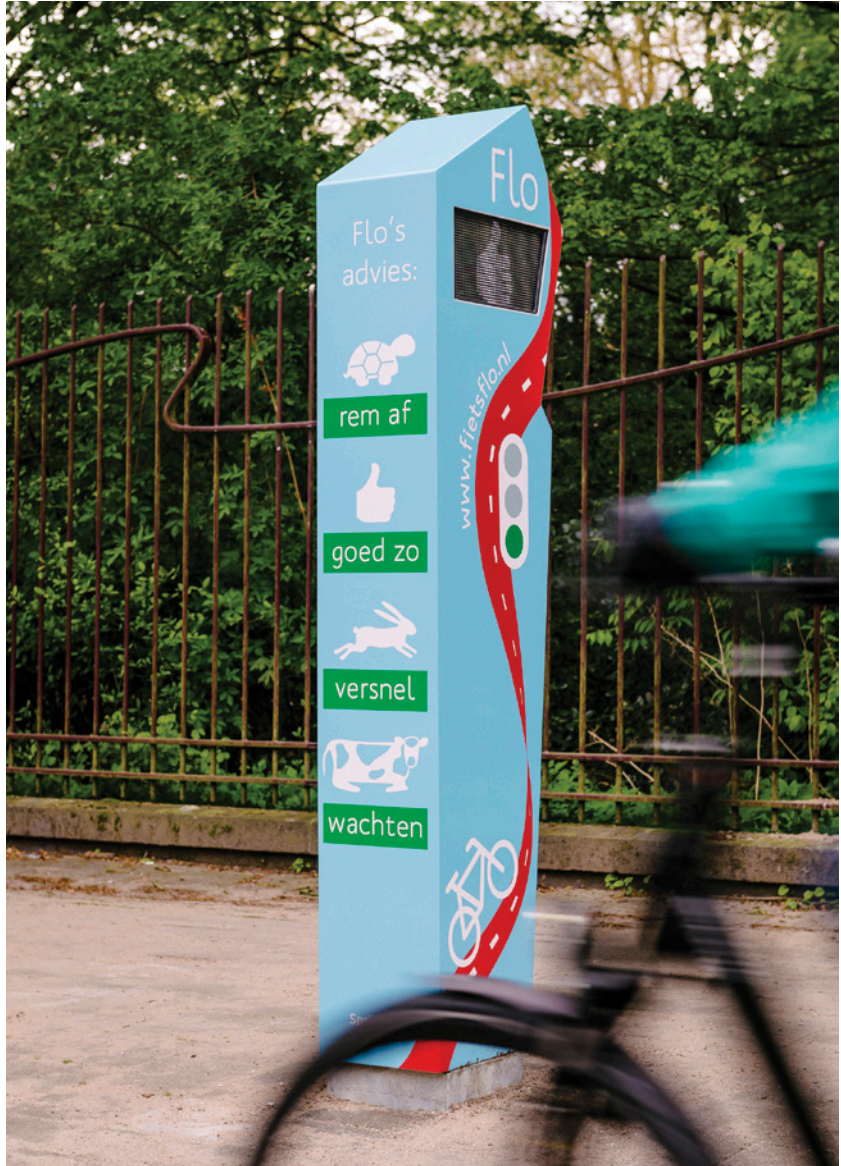
On the Amsterdamsstraatweg in Utrecht, the Flo system advises a cyclist to adjust his speed so that he can benefit from a 'green wave'.
