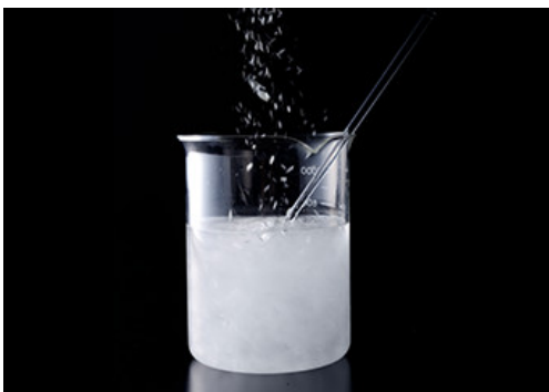
Figure 3 Wet chopped strands (Nippon Electric Glass Co., 2019)
