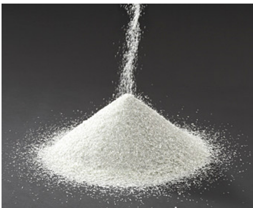
Figure 4 Dry chopped strands (Nippon Electric Glass Co., 2019)
