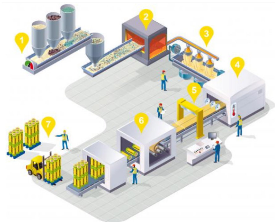
Figure 1 Glass wool manufacturing process (Isover Saint-Gobain, 2019)
