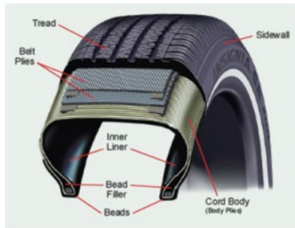
Figure 3 A simplified scheme of tyre components (V&F AUTO, 2016)
