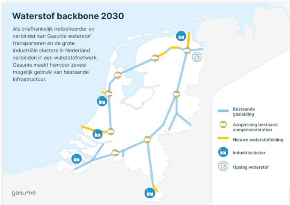
Figure 24 – Hydrogen Backbone infrastructure (Gasunie, 2020). Blue is existing gas pipeline, yellow is to-be-built hydrogen pipeline. The yellow symbols represent adaptations to existing compressor stations, the blue symbols are industry clusters and the light-blue symbol in the Northeast represents a hydrogen storage site.
