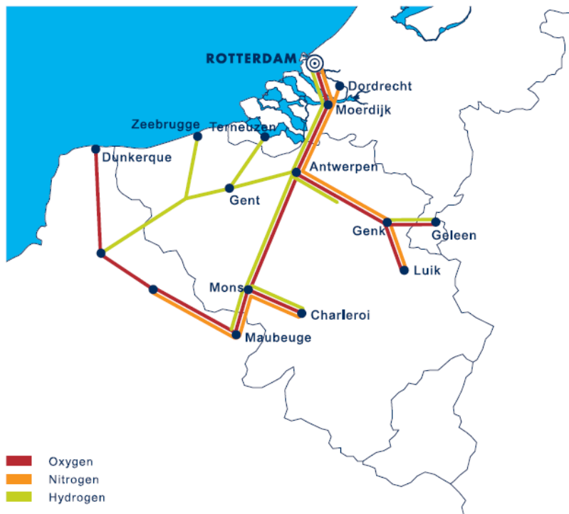
Figure 4 - Industrial gases pipelines (Port of Rotterdam, 2016)
