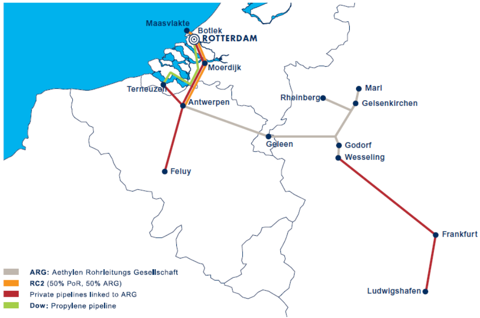
Figure 3 - Ethylene and propylene pipelines (Port of Rotterdam, 2016)
