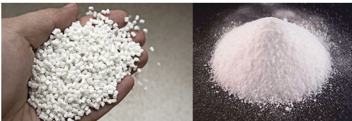
Figure 2. Bottle-grade PET (left) and PTA (right) at standard conditions.
