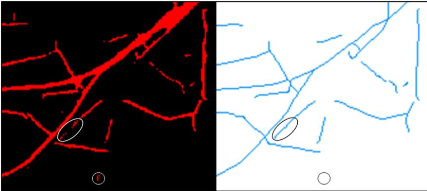
The figure shows two maps of post-processing, visualising the area around the hamlet of Marlboro in Canada. On the left: the model output in raster format. On the right: the model output after conversion into vector format with the centre line vectorisation method. Both maps have a small circle and a large circle showing the removal and connection of groups of pixels respectively.
