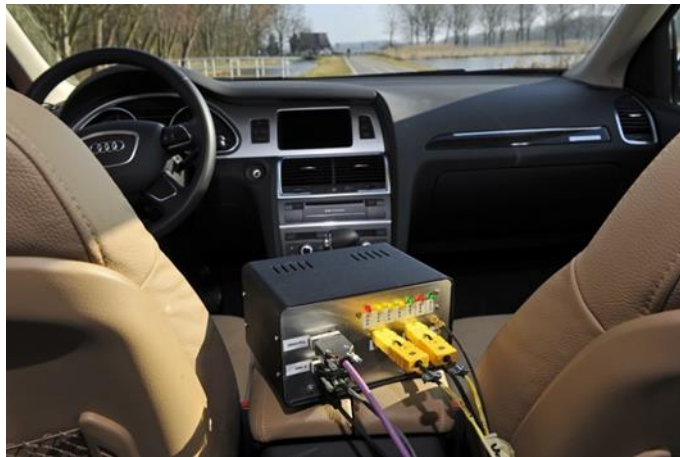
Figure 15: The SEMS system, developed by TNO, mounted on vehicles to be tested on the road (prototype version 2015).
