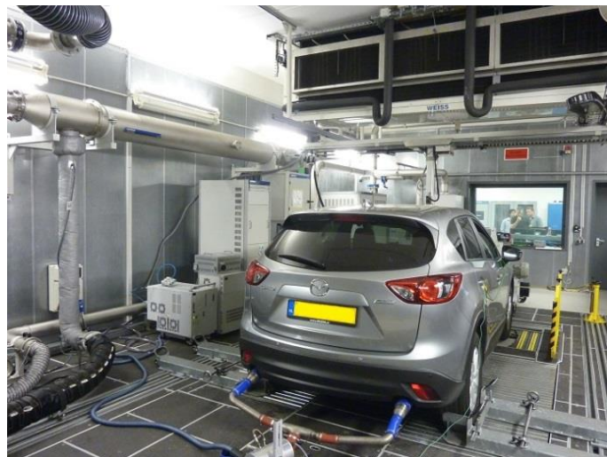
Figure 3: A passenger car tested in the laboratory on a two-wheel chassis dynamometer (roller bench).
