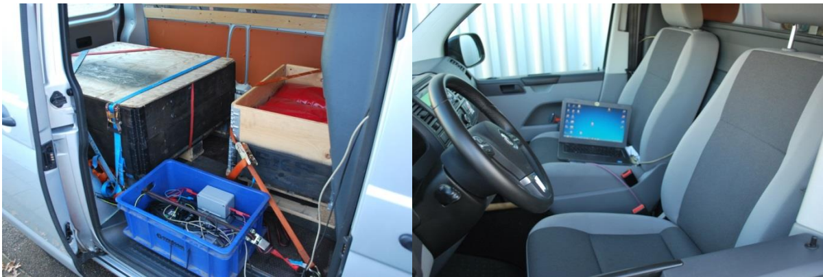
Figure 17: Left: Load packages (black box) and data logger of the SEMS (blue cradle) used in on-road testing of a light commercial vehicle. Right: The laptop used to monitor and control the SEMS equipment.
