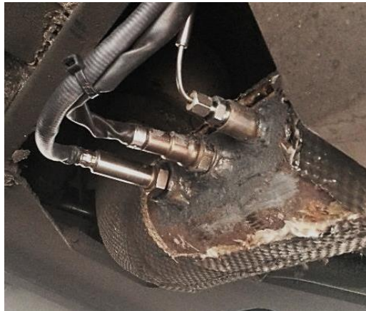
Figure 16: The SEMS sensors ( \text{NO}_x - \text{O}_2 , \text{NH}_3 and temperature) mounted in the exhaust.
